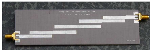
Figure 9: A microstrip filter designed using concatenated resonators. The connectors to the coax cable are the SMA (sub-miniature type A) connectors (Courtesy of aginas.fe.up.pt).
